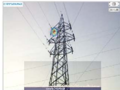
Discharge of insulators on 10kv transmission towers
