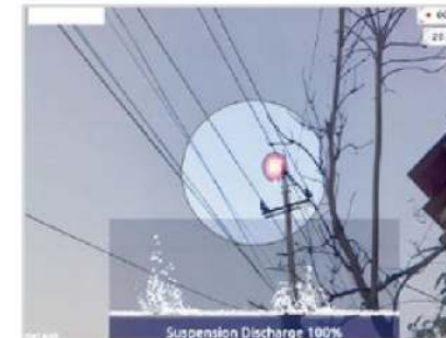
Discharge of insulators on 10kv tower poles
