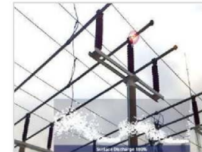
Discharge of porcelain bushings on outgoing lines
