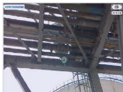
pipe welded seam leak
